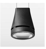
Suspended luminaire with LED, rated life of the LED L80/B10 > 50000 h, colour rendering index CRI > 90, chromaticity tolerance 2 SDCM (initial), reflector with oval light distribution pattern, reflector pure aluminium 99,99% in MIRO-Silver®, canopy sheet steel, powder-coated, luminaire head die-cast aluminium, powder-coated, stratoblack
