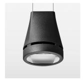
Suspended luminaire with LED, rated life of the LED L80/B10 > 50000 h, colour rendering index CRI > 90, chromaticity tolerance 2 SDCM (initial), reflector with oval light distribution pattern, reflector pure aluminium 99,99% in MIRO-Silver®, canopy sheet steel, powder-coated, luminaire head die-cast aluminium, powder-coated, stratoblack
