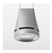
Suspended luminaire with LED, rated life of the LED L80/B10 > 50000 h, chromaticity tolerance 2 SDCM (initial), reflector with oval light distribution pattern, reflector pure aluminium 99,99% in MIRO-Silver®, canopy sheet steel, powder-coated, luminaire head die-cast aluminium, powder-coated, stratosilver
