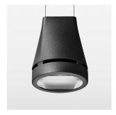
Suspended luminaire with LED, rated life of the LED L80/B10 > 50000 h, colour rendering index CRI > 80, chromaticity tolerance 2 SDCM (initial), reflector with oval light distribution pattern, reflector pure aluminium 99,99% in MIRO-Silver®, canopy sheet steel, powder-coated, luminaire head die-cast aluminium, powder-coated, stratoblack
