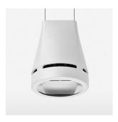
Suspended luminaire with LED, rated life of the LED L80/B10 > 50000 h, colour rendering index CRI > 90, chromaticity tolerance 2 SDCM (initial), reflector with oval light distribution pattern, reflector pure aluminium 99,99% in MIRO-Silver®, canopy sheet steel, powder-coated, luminaire head die-cast aluminium, powder-coated, stratowhite
