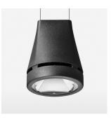
Suspended luminaire with LED, rated life of the LED L80/B10 > 50000 h, colour rendering index CRI > 80, chromaticity tolerance 2 SDCM (initial), reflector with circular light distribution pattern, reflector pure aluminium 99,99% in MIRO-Silver®, canopy sheet steel, powder-coated, luminaire head die-cast aluminium, powder-coated, stratoblack
