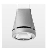
Suspended luminaire with LED, rated life of the LED L80/B10 > 50000 h, colour rendering index CRI > 80, chromaticity tolerance 2 SDCM (initial), reflector with circular light distribution pattern, reflector pure aluminium 99,99% in MIRO-Silver®, canopy sheet steel, powder-coated, luminaire head die-cast aluminium, powder-coated, stratosilver
