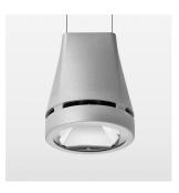
Suspended luminaire with LED, rated life of the LED L80/B10 > 50000 h, colour rendering index CRI > 90, chromaticity tolerance 2 SDCM (initial), reflector with circular light distribution pattern, reflector pure aluminium 99,99% in MIRO-Silver®, canopy sheet steel, powder-coated, luminaire head die-cast aluminium, powder-coated, stratosilver
