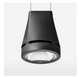
Suspended luminaire with LED, rated life of the LED L80/B10 > 50000 h, colour rendering index CRI > 90, chromaticity tolerance 2 SDCM (initial), reflector with circular light distribution pattern, reflector pure aluminium 99,99% in MIRO-Silver®, canopy sheet steel, powder-coated, luminaire head die-cast aluminium, powder-coated, stratoblack
