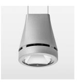
Suspended luminaire with LED, rated life of the LED L80/B10 > 50000 h, colour rendering index CRI > 80, chromaticity tolerance 2 SDCM (initial), reflector with circular light distribution pattern, reflector pure aluminium 99,99% in MIRO-Silver®, luminaire head die-cast aluminium, powder-coated, stratosilver, separate driver unit
