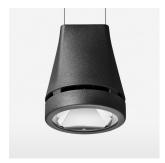
Suspended luminaire with LED, rated life of the LED L80/B10 > 50000 h, colour rendering index CRI > 90, chromaticity tolerance 2 SDCM (initial), reflector with circular light distribution pattern, reflector pure aluminium 99,99% in MIRO-Silver®, luminaire head die-cast aluminium, powder-coated, stratoblack, separate driver unit
