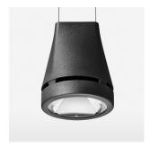
Suspended luminaire with LED, rated life of the LED L80/B10 > 50000 h, chromaticity tolerance 3 SDCM (initial), reflector with circular light distribution pattern, reflector pure aluminium 99,99% in MIRO-Silver®, luminaire head die-cast aluminium, powder-coated, stratoblack, separate driver unit
