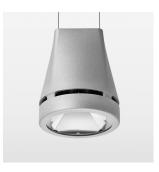
Suspended luminaire with LED, rated life of the LED L80/B10 > 50000 h, colour rendering index CRI > 90, chromaticity tolerance 2 SDCM (initial), reflector with circular light distribution pattern, reflector pure aluminium 99,99% in MIRO-Silver®, luminaire head die-cast aluminium, powder-coated, stratosilver, separate driver unit
