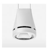
Suspended luminaire with LED, rated life of the LED L80/B10 > 50000 h, chromaticity tolerance 2 SDCM (initial), reflector with circular light distribution pattern, reflector pure aluminium 99,99% in MIRO-Silver®, luminaire head die-cast aluminium, powder-coated, stratowhite, separate driver unit
