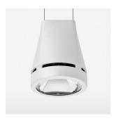
Suspended luminaire with LED, rated life of the LED L80/B10 > 50000 h, chromaticity tolerance 3 SDCM (initial), reflector with circular light distribution pattern, reflector pure aluminium 99,99% in MIRO-Silver®, luminaire head die-cast aluminium, powder-coated, stratowhite, separate driver unit
