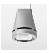
Suspended luminaire with LED, rated life of the LED L80/B10 > 50000 h, colour rendering index CRI > 90, chromaticity tolerance 2 SDCM (initial), reflector with circular light distribution pattern, reflector pure aluminium 99,99% in MIRO-Silver®, luminaire head die-cast aluminium, powder-coated, stratosilver, separate driver unit
