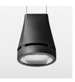
Suspended luminaire with LED, rated life of the LED L80/B10 > 50000 h, chromaticity tolerance 3 SDCM (initial), reflector with oval light distribution pattern, reflector pure aluminium 99,99% in MIRO-Silver®, luminaire head die-cast aluminium, powder-coated, stratoblack, separate driver unit
