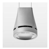
Suspended luminaire with LED, rated life of the LED L80/B10 > 50000 h, colour rendering index CRI > 90, chromaticity tolerance 2 SDCM (initial), reflector with oval light distribution pattern, reflector pure aluminium 99,99% in MIRO-Silver®, luminaire head die-cast aluminium, powder-coated, stratosilver, separate driver unit
