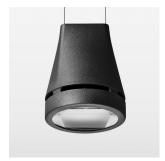
Suspended luminaire with LED, rated life of the LED L80/B10 > 50000 h, chromaticity tolerance 2 SDCM (initial), reflector with oval light distribution pattern, reflector pure aluminium 99,99% in MIRO-Silver®, luminaire head die-cast aluminium, powder-coated, stratoblack, separate driver unit
