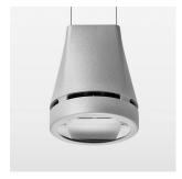
Suspended luminaire with LED, rated life of the LED L80/B10 > 50000 h, chromaticity tolerance 2 SDCM (initial), reflector with oval light distribution pattern, reflector pure aluminium 99,99% in MIRO-Silver®, luminaire head die-cast aluminium, powder-coated, stratosilver, separate driver unit
