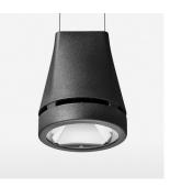
Suspended luminaire with LED, rated life of the LED L80/B10 > 50000 h, colour rendering index CRI > 80, chromaticity tolerance 2 SDCM (initial), reflector with circular light distribution pattern, reflector pure aluminium 99,99% in MIRO-Silver®, luminaire head die-cast aluminium, powder-coated, stratoblack, separate driver unit
