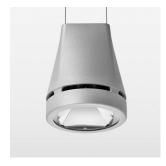
Suspended luminaire with LED, rated life of the LED L80/B10 > 50000 h, chromaticity tolerance 3 SDCM (initial), reflector with circular light distribution pattern, reflector pure aluminium 99,99% in MIRO-Silver®, luminaire head die-cast aluminium, powder-coated, stratosilver, separate driver unit
