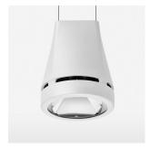
Suspended luminaire with LED, rated life of the LED L80/B10 > 50000 h, chromaticity tolerance 2 SDCM (initial), reflector with circular light distribution pattern, reflector pure aluminium 99,99% in MIRO-Silver®, luminaire head die-cast aluminium, powder-coated, stratowhite, separate driver unit
