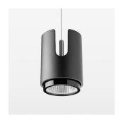
Suspended luminaire with LED, rated life of the LED L80/B10 > 50000 h, chromaticity tolerance 2 SDCM (initial), LED hybrid technology, 3D silicone lens to reduce the proportion of scattered light, reflector with circular light distribution pattern, reflector pure aluminium 99,99% in MIRO-Silver®, segmented and faceted, exchangeable reflector unit in high-sheen black plastic, with glass cover, luminaire housing die-cast aluminium, powder-coated, stratoblack, separate driver unit
