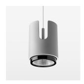
Suspended luminaire with LED, rated life of the LED L80/B10 > 50000 h, chromaticity tolerance 3 SDCM (initial), LED hybrid technology, 3D silicone lens to reduce the proportion of scattered light, reflector with circular light distribution pattern, reflector pure aluminium 99,99% in MIRO-Silver®, segmented and faceted, exchangeable reflector unit in high-sheen black plastic, with glass cover, luminaire housing die-cast aluminium, powder-coated, stratosilver, separate driver unit
