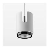
Suspended luminaire with LED, rated life of the LED L80/B10 > 50000 h, chromaticity tolerance 2 SDCM (initial), LED hybrid technology, 3D silicone lens to reduce the proportion of scattered light, reflector with circular light distribution pattern, reflector pure aluminium 99,99% in MIRO-Silver®, segmented and faceted, exchangeable reflector unit in high-sheen black plastic, with glass cover, luminaire housing die-cast aluminium, powder-coated, stratowhite, separate driver unit
