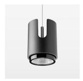
Suspended luminaire with LED, rated life of the LED L80/B10 > 50000 h, colour rendering index CRI > 96, chromaticity tolerance 3 SDCM (initial), , reflector with circular light distribution pattern, reflector pure aluminium 99,99% in MIRO-Silver®, segmented and faceted, exchangeable reflector unit in high-sheen black plastic, with glass cover, luminaire housing die-cast aluminium, powder-coated, stratoblack, separate driver unit
