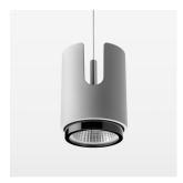
Suspended luminaire with LED, rated life of the LED L80/B10 > 50000 h, colour rendering index CRI > 80, chromaticity tolerance 2 SDCM (initial), , reflector with circular light distribution pattern, reflector pure aluminium 99,99% in MIRO-Silver®, segmented and faceted, exchangeable reflector unit in high-sheen black plastic, with glass cover, luminaire housing die-cast aluminium, powder-coated, stratosilver, separate driver unit
