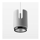
Suspended luminaire with LED, rated life of the LED L80/B10 > 50000 h, chromaticity tolerance 3 SDCM (initial), , reflector with circular light distribution pattern, reflector pure aluminium 99,99% in MIRO-Silver®, segmented and faceted, exchangeable reflector unit in high-sheen black plastic, with glass cover, luminaire housing die-cast aluminium, powder-coated, stratosilver, separate driver unit
