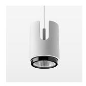
Suspended luminaire with LED, rated life of the LED L80/B10 > 50000 h, colour rendering index CRI > 90, chromaticity tolerance 2 SDCM (initial), , reflector with circular light distribution pattern, reflector pure aluminium 99,99% in MIRO-Silver®, segmented and faceted, exchangeable reflector unit in high-sheen black plastic, with glass cover, luminaire housing die-cast aluminium, powder-coated, stratowhite, separate driver unit
