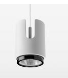
Suspended luminaire with LED, rated life of the LED L80/B10 > 50000 h, chromaticity tolerance 3 SDCM (initial), , reflector with circular light distribution pattern, reflector pure aluminium 99,99% in MIRO-Silver®, segmented and faceted, exchangeable reflector unit in high-sheen black plastic, with glass cover, luminaire housing die-cast aluminium, powder-coated, stratowhite, separate driver unit
