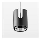
Suspended luminaire with LED, rated life of the LED L80/B10 > 50000 h, chromaticity tolerance 2 SDCM (initial), LED hybrid technology, 3D silicone lens to reduce the proportion of scattered light, reflector with oval light distribution pattern, reflector pure aluminium 99,99% in MIRO-Silver®, segmented, exchangeable reflector unit in high-sheen black plastic, with glass cover, luminaire housing die-cast aluminium, powder-coated, stratoblack, separate driver unit
