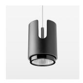
Suspended luminaire with LED, rated life of the LED L80/B10 > 50000 h, chromaticity tolerance 3 SDCM (initial), LED hybrid technology, 3D silicone lens to reduce the proportion of scattered light, reflector with oval light distribution pattern, reflector pure aluminium 99,99% in MIRO-Silver®, segmented, exchangeable reflector unit in high-sheen black plastic, with glass cover, luminaire housing die-cast aluminium, powder-coated, stratoblack, separate driver unit
