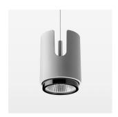
Suspended luminaire with LED, rated life of the LED L80/B10 > 50000 h, chromaticity tolerance 3 SDCM (initial), LED hybrid technology, 3D silicone lens to reduce the proportion of scattered light, reflector with oval light distribution pattern, reflector pure aluminium 99,99% in MIRO-Silver®, segmented, exchangeable reflector unit in high-sheen black plastic, with glass cover, luminaire housing die-cast aluminium, powder-coated, stratosilver, separate driver unit
