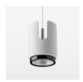
Suspended luminaire with LED, rated life of the LED L80/B10 > 50000 h, colour rendering index CRI > 90, chromaticity tolerance 2 SDCM (initial), LED hybrid technology, 3D silicone lens to reduce the proportion of scattered light, reflector with oval light distribution pattern, reflector pure aluminium 99,99% in MIRO-Silver®, segmented, exchangeable reflector unit in high-sheen black plastic, with glass cover, luminaire housing die-cast aluminium, powder-coated, stratowhite, separate driver unit
