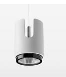
Suspended luminaire with LED, rated life of the LED L80/B10 > 50000 h, colour rendering index CRI > 96, chromaticity tolerance 3 SDCM (initial), LED hybrid technology, 3D silicone lens to reduce the proportion of scattered light, reflector with oval light distribution pattern, reflector pure aluminium 99,99% in MIRO-Silver®, segmented, exchangeable reflector unit in high-sheen black plastic, with glass cover, luminaire housing die-cast aluminium, powder-coated, stratowhite, separate driver unit
