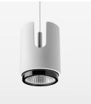
Suspended luminaire with LED, rated life of the LED L80/B10 > 50000 h, chromaticity tolerance 2 SDCM (initial), LED hybrid technology, 3D silicone lens to reduce the proportion of scattered light, reflector with oval light distribution pattern, reflector pure aluminium 99,99% in MIRO-Silver®, segmented, exchangeable reflector unit in high-sheen black plastic, with glass cover, luminaire housing die-cast aluminium, powder-coated, stratowhite, separate driver unit
