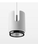
Suspended luminaire with LED, rated life of the LED L80/B10 > 50000 h, chromaticity tolerance 3 SDCM (initial), LED hybrid technology, 3D silicone lens to reduce the proportion of scattered light, reflector with oval light distribution pattern, reflector pure aluminium 99,99% in MIRO-Silver®, segmented, exchangeable reflector unit in high-sheen black plastic, with glass cover, luminaire housing die-cast aluminium, powder-coated, stratowhite, separate driver unit
