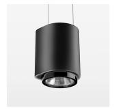
Suspended luminaire with LED, rated life of the LED L80/B10 > 50000 h, colour rendering index CRI > 80, chromaticity tolerance 2 SDCM (initial), LED hybrid technology, 3D silicone lens to reduce the proportion of scattered light, reflector with circular light distribution pattern, reflector pure aluminium 99,99% in MIRO-Silver®, segmented and faceted, exchangeable reflector unit in high-sheen black plastic, with glass cover, luminaire housing die-cast aluminium, powder-coated, stratoblack
