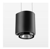
Suspended luminaire with LED, rated life of the LED L80/B10 > 50000 h, chromaticity tolerance 3 SDCM (initial), LED hybrid technology, 3D silicone lens to reduce the proportion of scattered light, reflector with circular light distribution pattern, reflector pure aluminium 99,99% in MIRO-Silver®, segmented and faceted, exchangeable reflector unit in high-sheen black plastic, with glass cover, luminaire housing die-cast aluminium, powder-coated, stratoblack, separate driver unit
