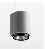
Suspended luminaire with LED, rated life of the LED L80/B10 > 50000 h, colour rendering index CRI > 80, chromaticity tolerance 2 SDCM (initial), LED hybrid technology, 3D silicone lens to reduce the proportion of scattered light, reflector with circular light distribution pattern, reflector pure aluminium 99,99% in MIRO-Silver®, segmented and faceted, exchangeable reflector unit in high-sheen black plastic, with glass cover, luminaire housing die-cast aluminium, powder-coated, stratosilver
