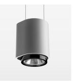
Suspended luminaire with LED, rated life of the LED L80/B10 > 50000 h, chromaticity tolerance 2 SDCM (initial), LED hybrid technology, 3D silicone lens to reduce the proportion of scattered light, reflector with circular light distribution pattern, reflector pure aluminium 99,99% in MIRO-Silver®, segmented and faceted, exchangeable reflector unit in high-sheen black plastic, with glass cover, luminaire housing die-cast aluminium, powder-coated, stratosilver, separate driver unit
