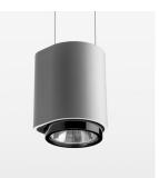
Suspended luminaire with LED, rated life of the LED L80/B10 > 50000 h, chromaticity tolerance 3 SDCM (initial), LED hybrid technology, 3D silicone lens to reduce the proportion of scattered light, reflector with circular light distribution pattern, reflector pure aluminium 99,99% in MIRO-Silver®, segmented and faceted, exchangeable reflector unit in high-sheen black plastic, with glass cover, luminaire housing die-cast aluminium, powder-coated, stratosilver, separate driver unit
