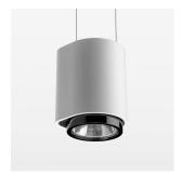
Suspended luminaire with LED, rated life of the LED L80/B10 > 50000 h, colour rendering index CRI > 96, chromaticity tolerance 3 SDCM (initial), LED hybrid technology, 3D silicone lens to reduce the proportion of scattered light, reflector with circular light distribution pattern, reflector pure aluminium 99,99% in MIRO-Silver®, segmented and faceted, exchangeable reflector unit in high-sheen black plastic, with glass cover, luminaire housing die-cast aluminium, powder-coated, stratowhite
