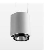
Suspended luminaire with LED, rated life of the LED L80/B10 > 50000 h, chromaticity tolerance 2 SDCM (initial), LED hybrid technology, 3D silicone lens to reduce the proportion of scattered light, reflector with circular light distribution pattern, reflector pure aluminium 99,99% in MIRO-Silver®, segmented and faceted, exchangeable reflector unit in high-sheen black plastic, with glass cover, luminaire housing die-cast aluminium, powder-coated, stratowhite
