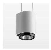
Suspended luminaire with LED, rated life of the LED L80/B10 > 50000 h, chromaticity tolerance 2 SDCM (initial), LED hybrid technology, 3D silicone lens to reduce the proportion of scattered light, reflector with circular light distribution pattern, reflector pure aluminium 99,99% in MIRO-Silver®, segmented and faceted, exchangeable reflector unit in high-sheen black plastic, with glass cover, luminaire housing die-cast aluminium, powder-coated, stratowhite
