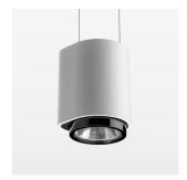
Suspended luminaire with LED, rated life of the LED L80/B10 > 50000 h, chromaticity tolerance 2 SDCM (initial), LED hybrid technology, 3D silicone lens to reduce the proportion of scattered light, reflector with circular light distribution pattern, reflector pure aluminium 99,99% in MIRO-Silver®, segmented and faceted, exchangeable reflector unit in high-sheen black plastic, with glass cover, luminaire housing die-cast aluminium, powder-coated, stratowhite, separate driver unit
