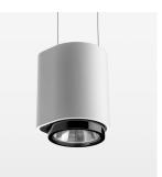
Suspended luminaire with LED, rated life of the LED L80/B10 > 50000 h, chromaticity tolerance 3 SDCM (initial), LED hybrid technology, 3D silicone lens to reduce the proportion of scattered light, reflector with circular light distribution pattern, reflector pure aluminium 99,99% in MIRO-Silver®, segmented and faceted, exchangeable reflector unit in high-sheen black plastic, with glass cover, luminaire housing die-cast aluminium, powder-coated, stratowhite, separate driver unit
