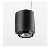
Suspended luminaire with LED, rated life of the LED L80/B10 > 50000 h, colour rendering index CRI > 80, chromaticity tolerance 2 SDCM (initial), , reflector with circular light distribution pattern, reflector pure aluminium 99,99% in MIRO-Silver®, segmented and faceted, exchangeable reflector unit in high-sheen black plastic, with glass cover, luminaire housing die-cast aluminium, powder-coated, stratoblack, separate driver unit
