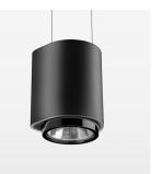
Suspended luminaire with LED, rated life of the LED L80/B10 > 50000 h, colour rendering index CRI > 80, chromaticity tolerance 2 SDCM (initial), , reflector with circular light distribution pattern, reflector pure aluminium 99,99% in MIRO-Silver®, segmented and faceted, exchangeable reflector unit in high-sheen black plastic, with glass cover, luminaire housing die-cast aluminium, powder-coated, stratoblack
