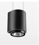
Suspended luminaire with LED, rated life of the LED L80/B10 > 50000 h, colour rendering index CRI > 90, chromaticity tolerance 2 SDCM (initial), , reflector with circular light distribution pattern, reflector pure aluminium 99,99% in MIRO-Silver®, segmented and faceted, exchangeable reflector unit in high-sheen black plastic, with glass cover, luminaire housing die-cast aluminium, powder-coated, stratoblack, separate driver unit
